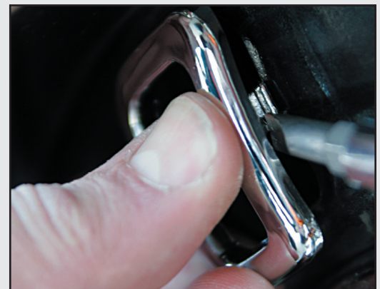
Figure 1B: Gently Nudge other tab with screwdriver
