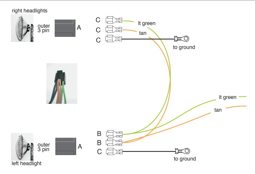
The 1970 Mustang utilized a single headlamp system as opposed to the dual headlamp system used on the 1969 Mustangs. On this sheet, you will find instructions that depict how to connect your headlamps. The function of each of the wires (It. green, tan, and black) remains the same as on the main instruction sheet 510178, page 2, branch 2. AAW recommends that you use both this sheet and the 510178 sheet for installation of your headlamps.
